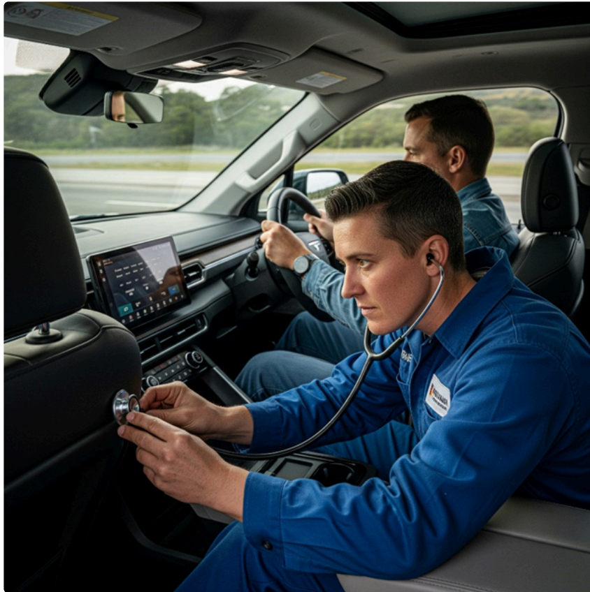
Figure 10. Using a Stethoscope While Driving
