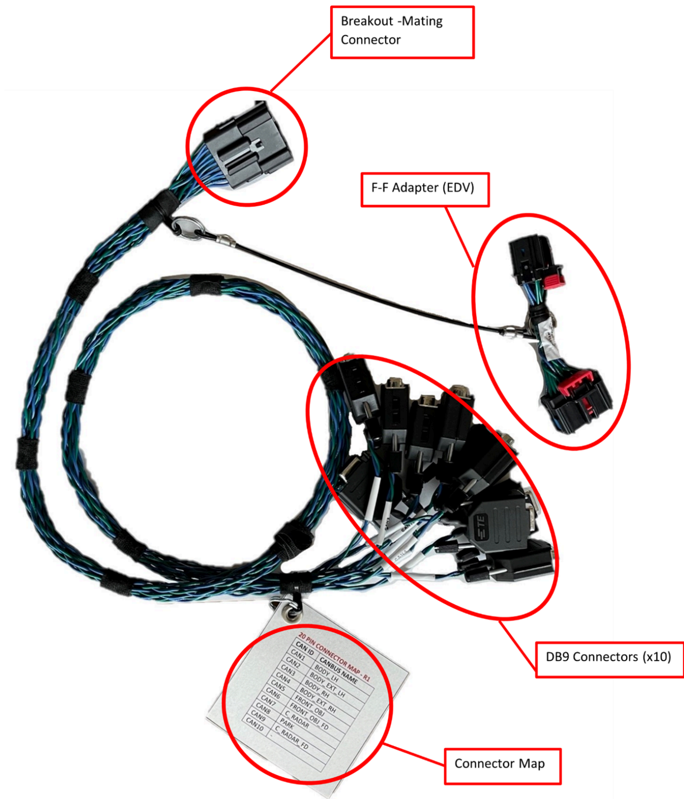
Figure 46. CAN Breakout Interface Box
