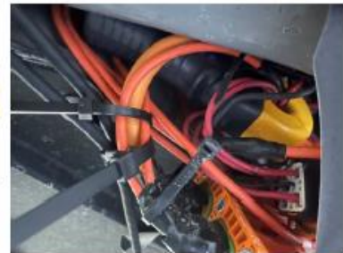
DC/DC Converter, AC Compressor & On-Board Charger – 200A
