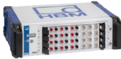
Above: Hioki CT684X-05 current clamp and HBM Gen4TB power analyzer
