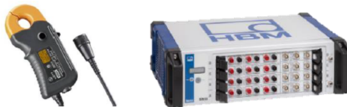
Above: Hioki CT684X-05 current clamp and HBM Gen4TB power analyzer
